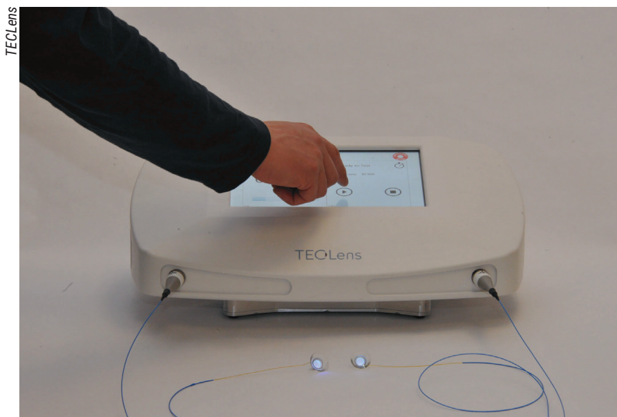
The CXLens platform includes a compact system with lenses that emit UV-A light rays for cross-linking treatment. Two lenses are attached to the device to perform cross-linking on both eyes simultaneously.
