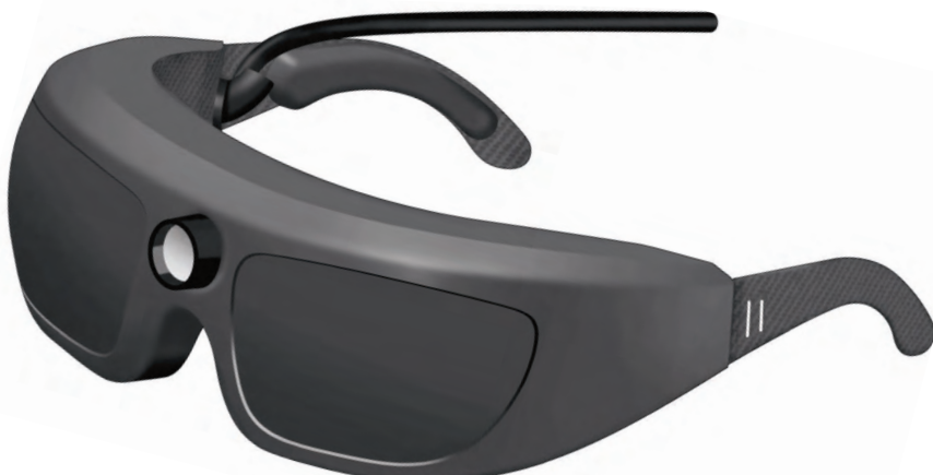
A prototype design of GenSight Biologics' GS030-MD goggles. According to GenSight, the front of the product features a camera which captures the natural environment and sends a stream of images to a projector inside the device. A cable runs down the side of the device and connects to a processing unit with software that alters the images to the correct light intensity.
