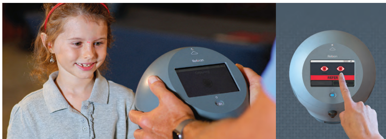
The Blinq Pediatric Vision Scanner (Rebion) detects abnormal bifoveal fixation as small as one degree. The device provides a “pass” or “refer” signal after testing. Unlike traditional amblyopia screening tests, Blinq has a low false-positive rate, the company says.
