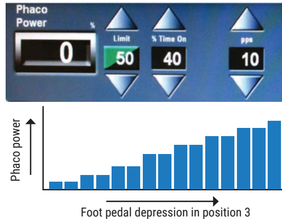
Figure 2. In phaco pulse mode, the time between pulses, known as the off time, allows the phaco needle to cool, reducing the heat and energy delivered into the eye.
