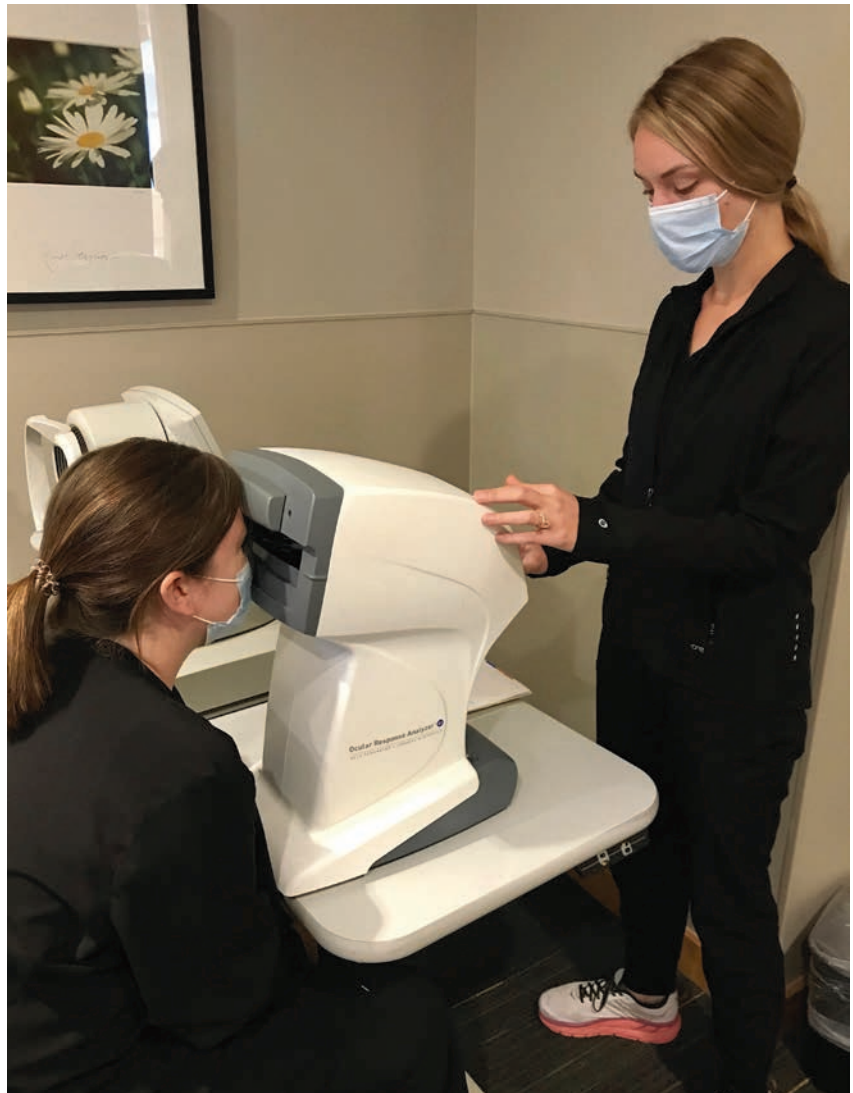
A technician in Dr. Berdahl's office measures a patient's corneal hysteresis. Dr. Berdahl routinely measures hysteresis in all patients.
