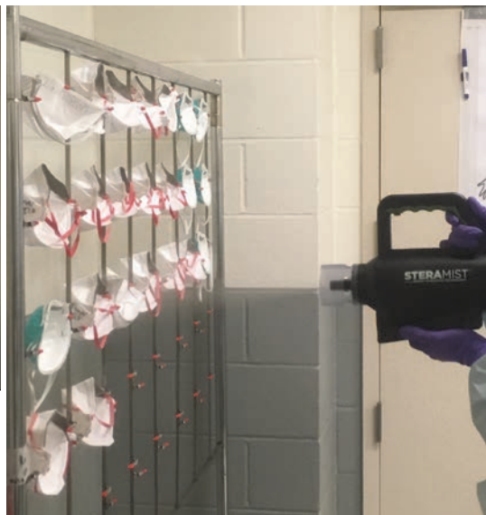
Vaporized hydrogen peroxide is effective against coronavirus, although it can be toxic at high concentrations. Above: The SteraMist device ionizes a lower-concentration hydrogen peroxide mist by passing it through a 17,000-volt electric arc; the resulting ions destroy bacteria and viruses without harming materials or electronics. Right: The device is used to mist surgical masks.
