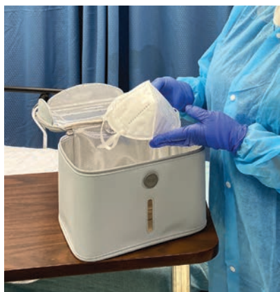
Ultraviolet-C light has been proven to kill the coronavirus, given sufficient exposure. Here, a box containing multiple UV-C lamps is used to sterilize a surgical mask by irradiating it from all sides for 10 minutes.
