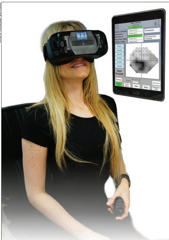
A limitation of using portable devices to perform VF testing is the inability to control fixation and the distance from the eye to the screen. Virtual reality headsets may solve those issues through adjustable fixation using gaze tracking.
