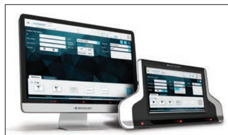
The EyeSwift system uses eyetracking to evaluate the vision of a child (or adult) while the subject watches an entertaining video. (See illustration, facing page.)
