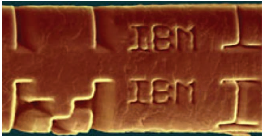
Unmatched precision: The excimer laser was once used to carve the IBM company logo onto a human hair. The femtosecond is incapable of such feats, Dr. Wilson says.
