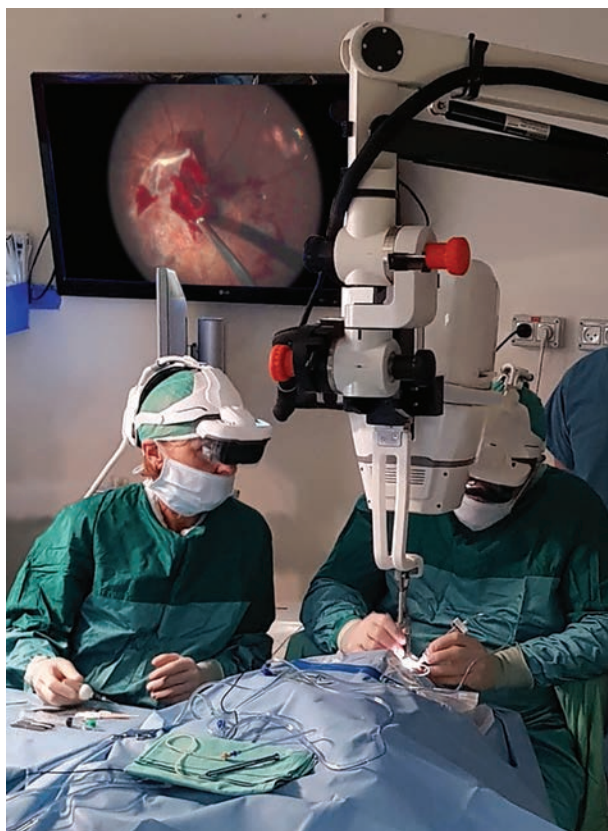
Figure 1. Diabetic retinopathy case. The dual 3-D ultra resolution cameras are suspended on a remote arm. The surgeon and the assistant wear transparent head-mounted displays that allow information to flow toward them in high resolution.
