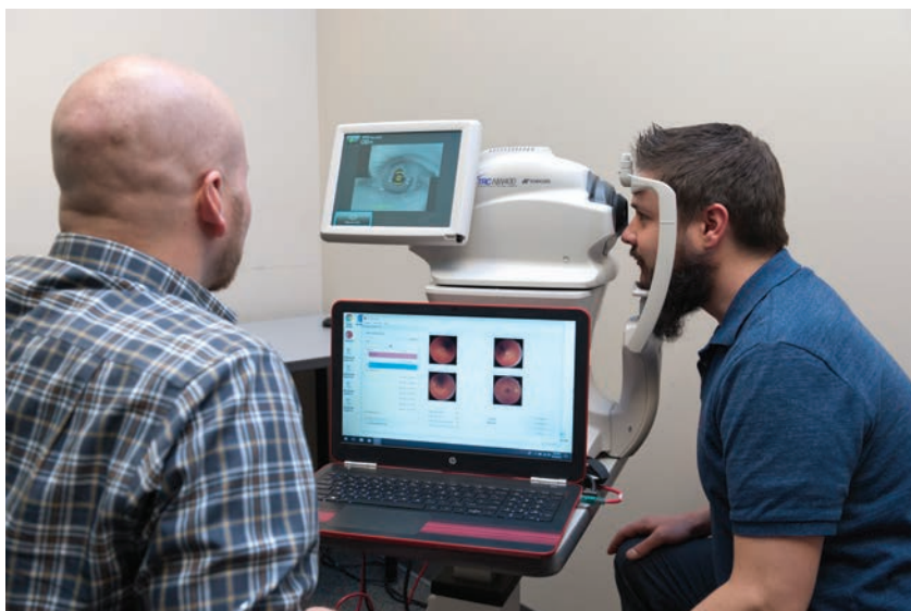
The IDx-DR was able to successfully produce a disease evaluation for 96 percent of subjects in a clinical trial, with fewer than a quarter of them needing dilation. The artificial intelligence built into the device helps ensure that the operator gets high-quality images.
