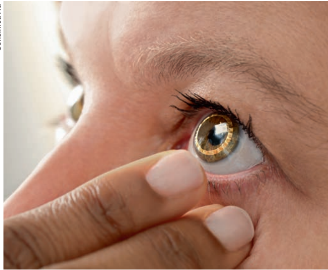
The Triggerfish contact lens sensor, shown here without the receiver taped around the orbit, has tiny strain gauges and telemetry circuits embedded inside.
