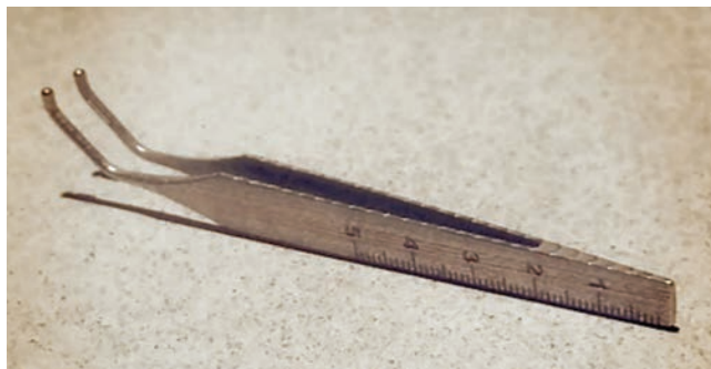
A new tool can be designed (left) and 3-D printed (above) in small quantities for a reasonable price, allowing testing in the clinic, leading to improved versions without involving a major manufacturer.
