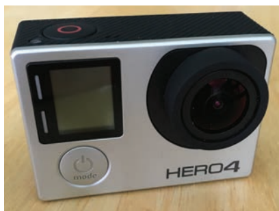
Figure 4. The GoPro Hero4 Silver Edition. GoPro is worn on the forehead of the surgeon with the camera mounted on a head strap within a case. The compact camera is equipped with a touchscreen display, micro-speaker, and Wi-Fi. It records in 1080p and takes 12 MP still shots.
