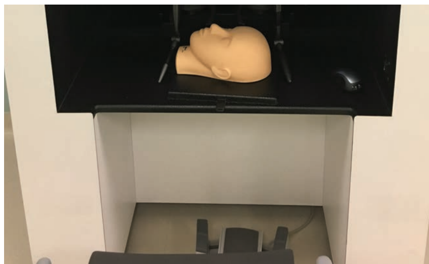
The MicroVisTouch cataract surgery simulator has foot pedals that allow trainees to practice the phacoemulsification step.
