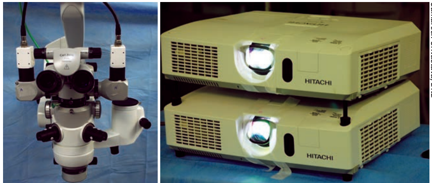
Above, left: Two similar cameras mounted on either side of a microscope’s beam splitter using video adapter tubes of the same focal length. Above, right: Two stackable projectors with their projected images aligned. A pair of polarized eyeglasses has been broken in half, with one lens placed in front of each projector’s lens to polarize the projected images.
