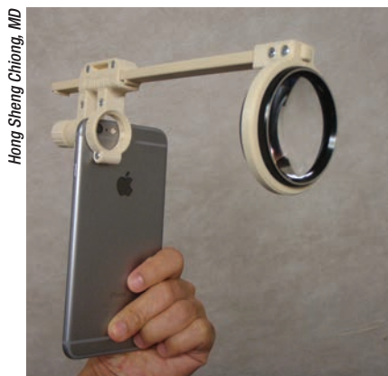
The OphthalmicDocs Fundus is inexpensive because you make it on a 3D printer.
