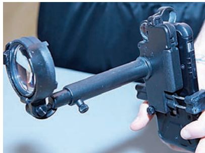
Smartphone technology is helping to make eye examinations more portable. Above: the Paxos Scope (DigiSight Technologies), a universal smartphone adapter that allows doctors to capture high-resolution anterior and posterior images of the eye.
