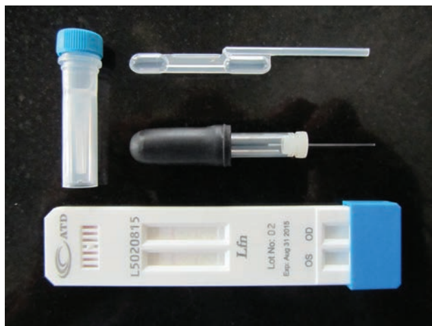
Advanced Tear Diagnostics' TearScan system measures levels of lactoferrin, associated with the level of aqueous tear production, as well as the level of IgE, an allergy-related marker. A sample is placed into the vial (left) for dilution; the pipette at the top transfers the correct amount of fluid to the test cassette. The cassette is inserted into the TearScan Reader to get numeric results.
