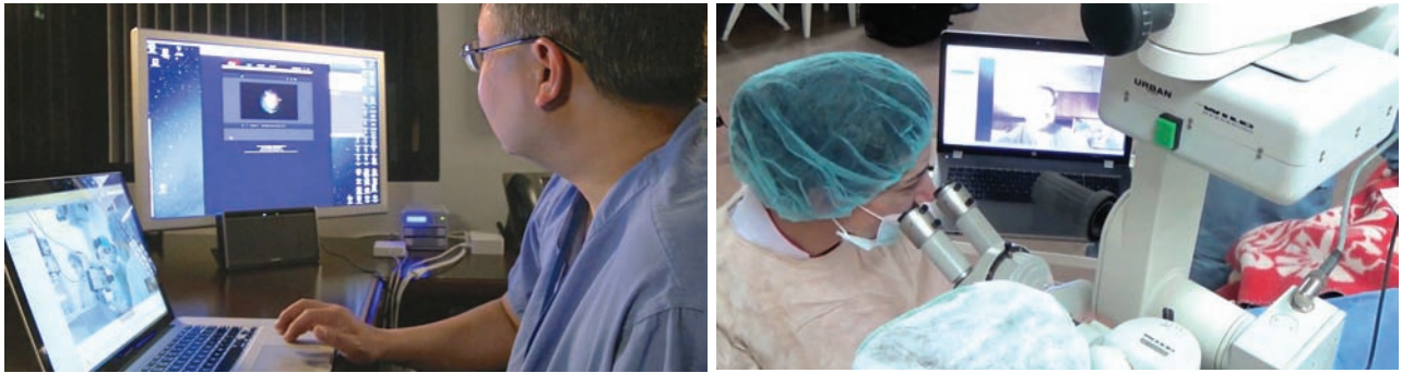
The interactive video setup designed by Thomas C. Lee, MD, uses Skype on one computer screen for communicating with the remote surgeons while the endoscopic surgical image appears on a separate screen, transmitted via the Slingbox, designed for use with cable television.
