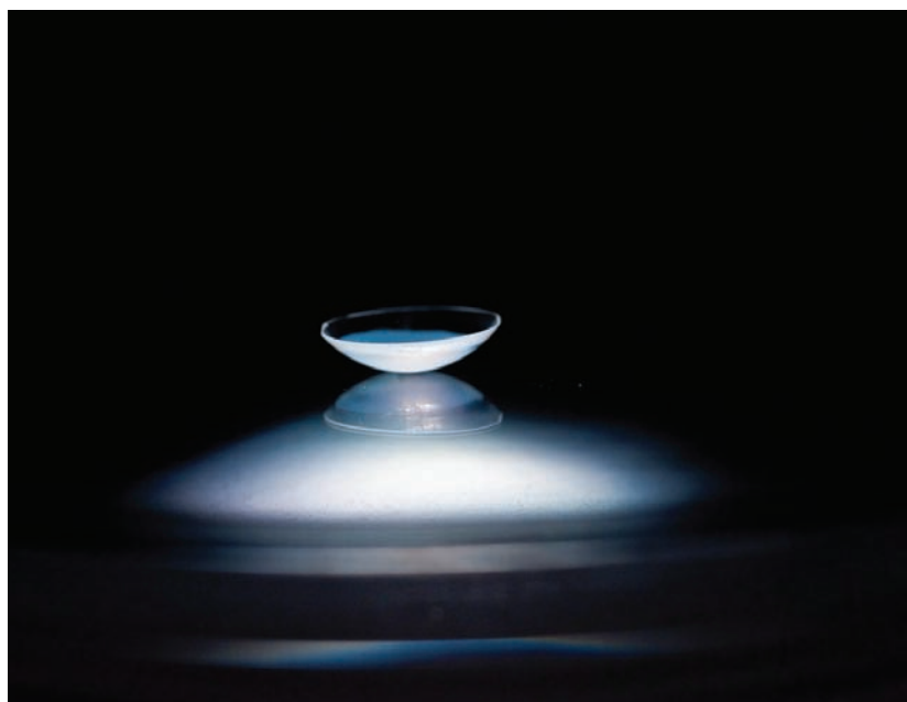
A new contact lens prototype releases drugs fairly evenly for 30 days or longer, while also correcting refractive error. Human trials of the lens should begin soon.
