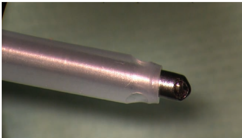
The Cetus nano laser phaco system houses a laser in the tip. The laser strikes a titanium target, and the resulting shockwaves emulsify the nuclear material.
