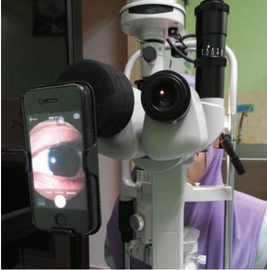
This slit-lamp adapter, designed by a surgeon in Malaysia, can be assembled in a few minutes from parts costing about $15. It slides onto the slit lamp eye piece (left) allowing a tech or surgeon to capture images like those above.
